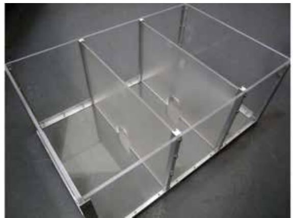
Figure 1. The 3-chamber apparatus used for testing innate aversion. Experimental stimuli can be presented in either side chamber of the apparatus. The mouse begins the trial in the center chamber; after a 10-min acclimation period, removable door panels are lifted, allowing exploration of both side chambers. This image shows the apparatus with the door panels removed, exposing 2 holes in the interior walls that allow mice to travel freely between the chambers.
